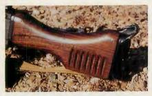
FN MAG 58's distinctive wooden buttstock houses the "hard" buffer with 11 Bellville washers required for a high cyclic-rate machine gun.
